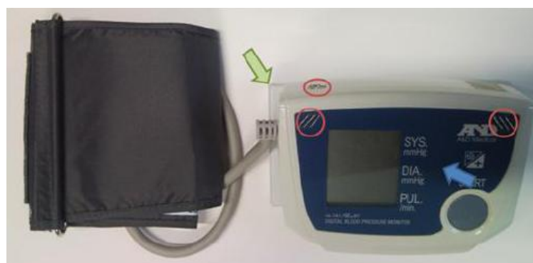
Figure 2: Extended blood pressure meter. The left arrow marks the attached case; the right arrow indicates the position of the RFID tag, the red circles mark the three metal electrodes to be touched by the patient with her/his fingers.
