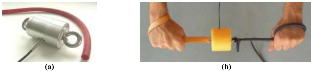
Figure 5: Force sensor (a) force sensor with case and (b) mounted on the band.
