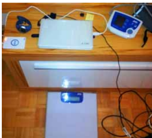
Figure 2: Patient environment consisting of a data hub (netbook), smart card reader, blood pressure meter, weight scale and sports watch
